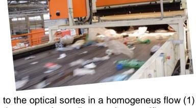
Wastes arrive to the optical sortes in a homogeneus flow (1) and the optical sorters, depending on the specific set-up, can locate the exact position of each fraction that have to be recovered/rejected (2).
